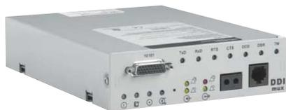
Digital Drop and Insert Mux (DDIM)
